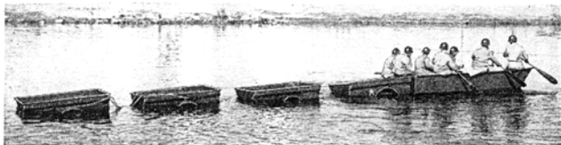
Figure 9.—Four \frac{1}{4} -ton trailers containing a 500-pound, evenly distributed load towed by M2 assault boat with seven men paddling and one man steering.
